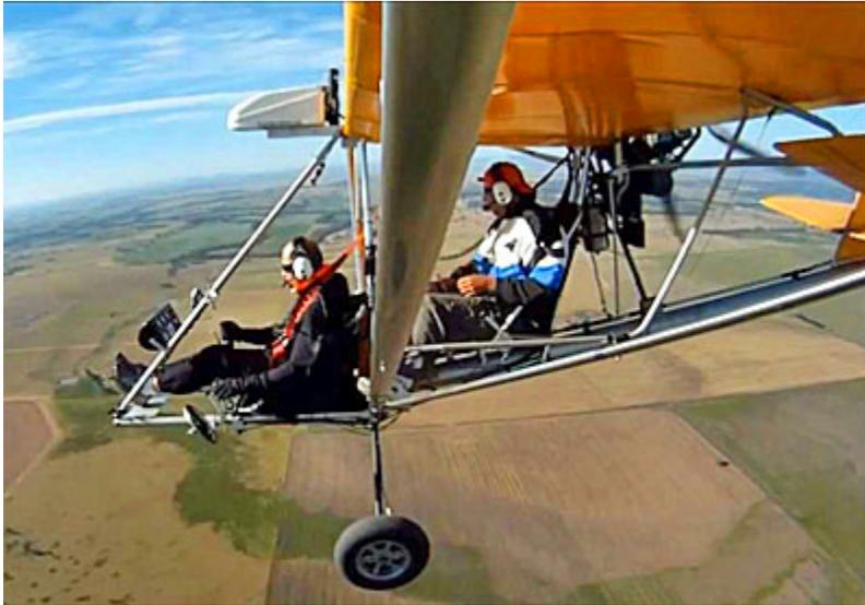
I asked Ed to explain what they did to bump gross and Vne speed. "We reduced rudder pressure, added electric flaperons, reinforced the main gear, and improved longitudinal stability of the Dragonfly," he clarified. A nose cone and windscreen reduces fatigue for a working pilot. Yet Dragonfly remains "fun to fly," he assured. "It actually performs better with flaps up in aerobatics — spins and loops — and still does a controllable flat spin."
