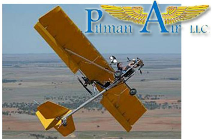
Note the tall mast extending from the vertical stabilizer; another component can be seen aft of the tailwheel. This is part of the tow bridle system used to safely tow hang gliders.
